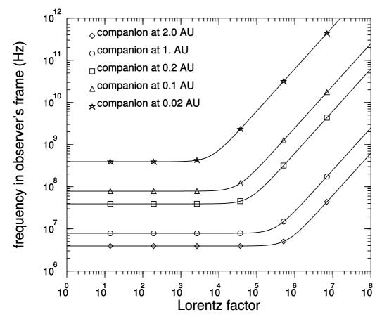
Fig. 6. Cyclotron frequency in the observer's frame as a function of the pulsar wind Lorentz factor  $\gamma$ , from Eq. (16) for various distances of the companion. Values that are not varied are the same as in the text: the magnetic field is  $B_* = 10^5$  T and the spin period  $T_* = 10$  ms.
